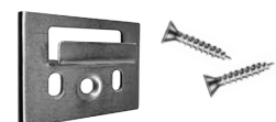
Metal clips for installation of slatted wall cladding. 3pcs per 1m board (screws supplied)
